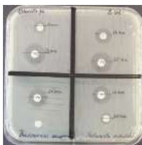
Figure 1. Testing the phytocomplex by diffusimetric method against Escherichia coli ATCC 25922, Pseudomonas aeruginosa ATCC 27853, Salmonella enterica ATCC 13076, Klebsiella pneumoniae ATCC ATCC 13883. Muller Hinton agar medium, Gentamicin (Gn / 10 µg)
