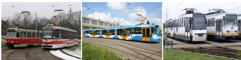
Fig. 1 – Tatra T3 / Tatra K2 / V3A93 tram modernization, became V3A93CHPPC (photographs source – www.tramclub.ro )
