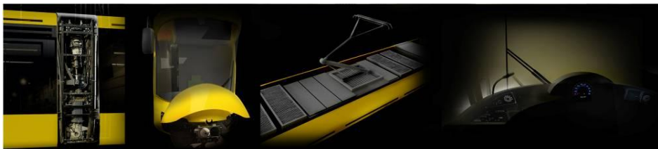
Fig. 4. Vertical placement of the motors / Coupling system / Pantograph/ Dashboard.
