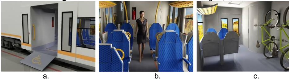
Fig. 11. Modernized wagon concept: a. Access ramp for people with disabilities; b. Interior; c. Bicycle supports
