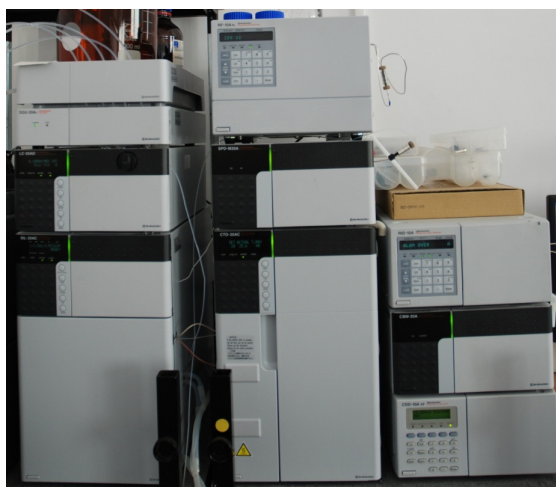
Fig. 1 - HPLC system used in the determination of phenolic acids
