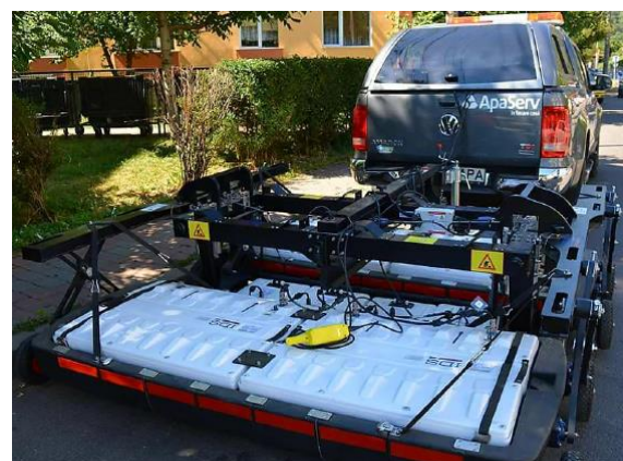
Figure 9. Pipe detection equipment type Georadar
