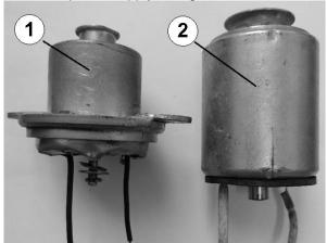
Figure 3 Electromagnets used on the test stand 1- Type 1 electromagnet; 2 – Type 2 electromagnet.
