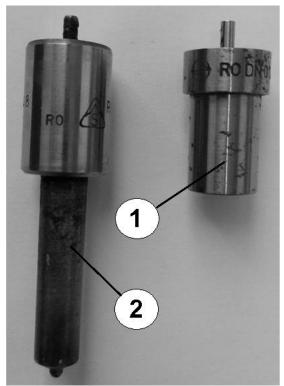
Figure 4 **Injector sprayers used on the test stand** 1- Type A sprayer; 2 sprayer – Type B.
