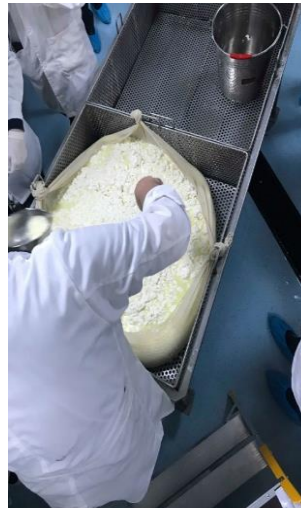
Figure 8 Transfer of the coagulum into the ridge
