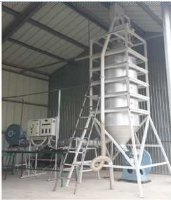
Figure 7: Innovation vertical drier with heat recovery
