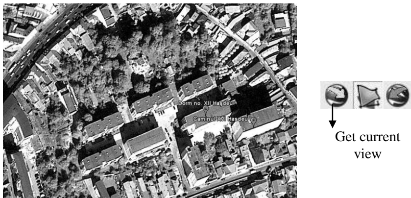
Fig. 1. Selection of the studied area in Google Earth and its importing protocol in Google SketchUP using Get current view function
