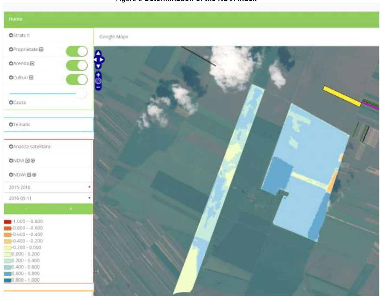
Figure 7 Determination of the NDWI index - the water level in the plant
