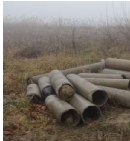
Figure 7 Condition of degradation of asbestos pipes in the structure of the pipeline network of "Berezeni Plot 16" (Luca, 2015)
