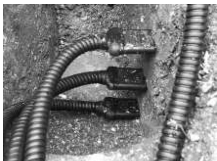
Figure 9 Three level soil moisture measuring (site #3)
