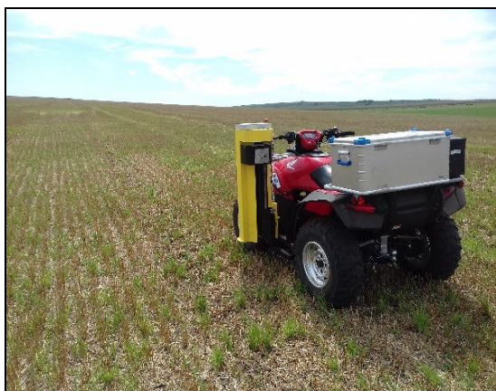
Figure 2 Soil agrochemical sampling set-up
