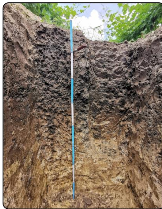
Figure 1 Soil profile – cerno-cambic aric anthrosol
