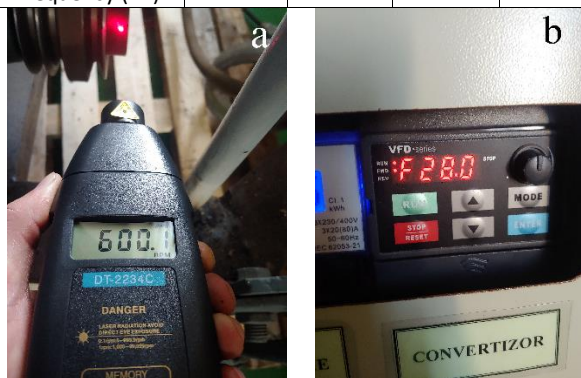
Figure 2 Frequency setting versus fan speed
