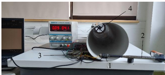
Figure 4 Stand for calibrating the air flow velocity sensor
