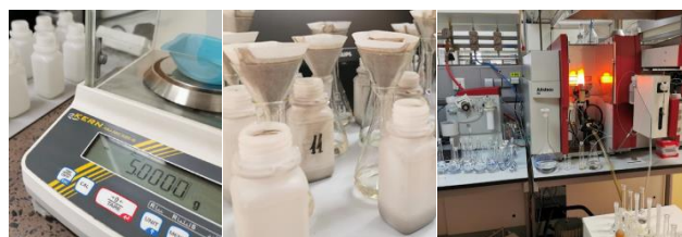
Figure 3 Micronutrients extraction with atomic adsorption spectrometer
