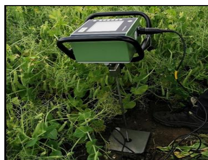
Figure 2 Determination of soil penetration resistance
