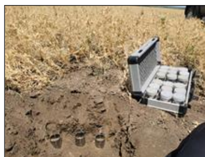
Figure 1 Bulk density sampling
