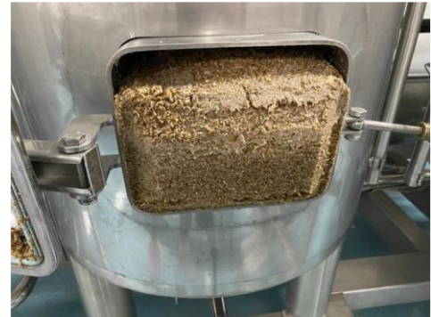
Figure 8. Disposal of slurry malt
