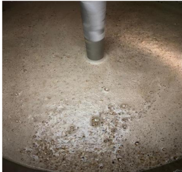
Figure 6. Immersing the malt grind in water
