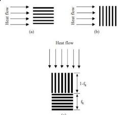
Figure 4 Models for the calculation of heat conductivity
