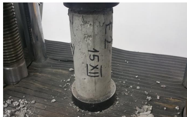
Figure 1 Experimental test in compression of concrete with polystyrene granules
