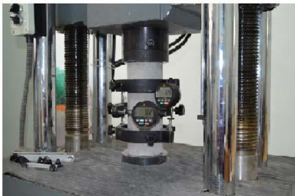
Figure 1 Experimental test in compression of concrete with polystyrene granules
