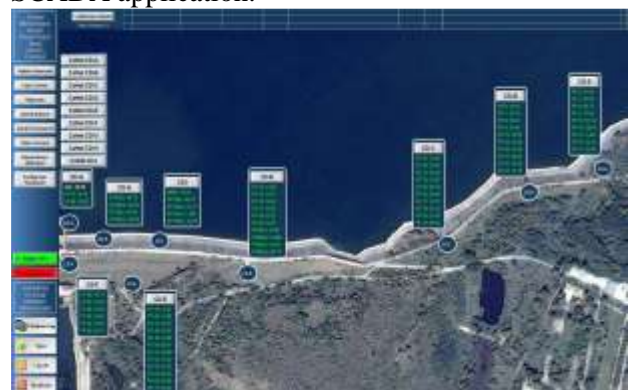
Figure 10. The main screen of the soft SCADA
