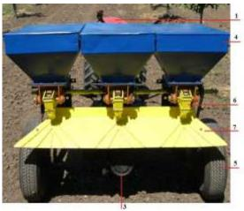
Fig. 1 **Solid chemical fertilizer equipment**: **a** – *lateral view*; **b** – *back view*; 1 – motocultor; 2 – chassis;
