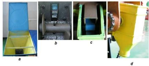
Fig. 2. **Work section** (*details*): **a** – fertilizer box; **b** – rotative stirrer; **c** – distributor; **d** – driving tube.
