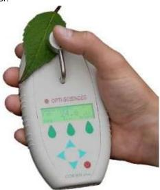
Figure1 Device used for determining the chlorophyll content of leaves (http://www.envcoglobal.com)
