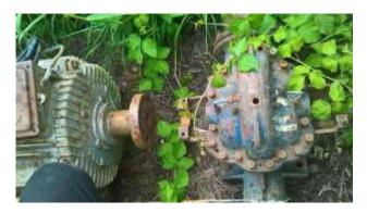
Figure 4 SPPM 7/7-2 pump aggregates status (RDN 200-150-200 pump and motor) (Photo Luca M., 2016)
