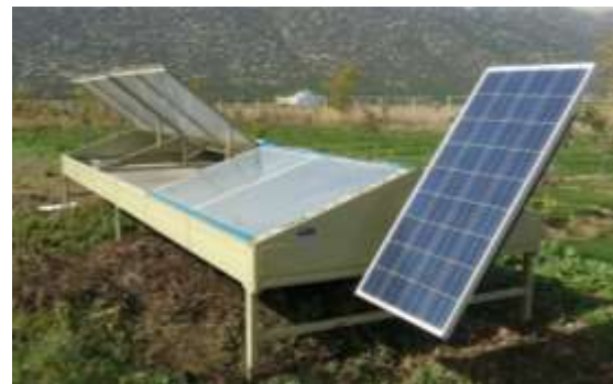
Figure 1 The experimental solar tunnel dryer
