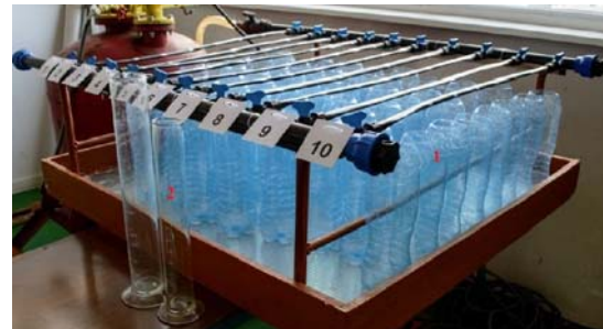
Figure 2 Experimental stand 1 – plastic container; 2 – cylinder; N – drainer
