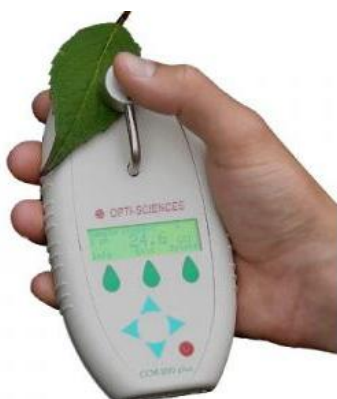
Figure 2 Device for determining the chlorophyll content of leaves ( http://www.envcoglobal.com )
