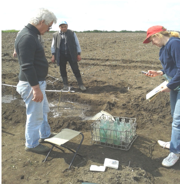
Figure 3 Determining the volume and turbidity leaks under the influence of artificial rain of certain intensity
