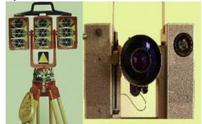
Figure 5 Geodetic Distance Meter - Model 6 Geodimeter with batery of nine prisms
