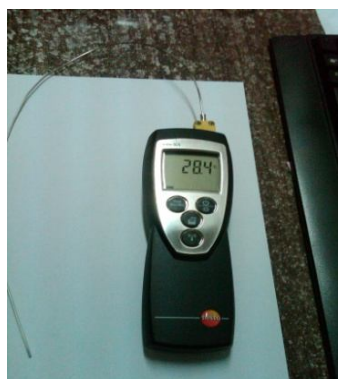
Figure 2 Devices for measuring the temperature and velocity the drying agent a - anemometer, b - type K thermocouple thermometer
