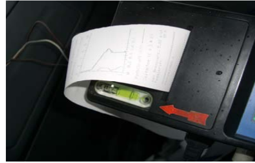
Figura 5b Decelerometer used on vehicles without ABS
