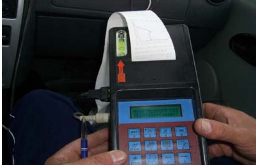
Figura 5a Decelerometer used on vehicles with ABS
