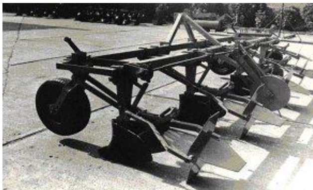
Figure 1 DBM-5 with the equipment used for making divided furrows on sloping lands
