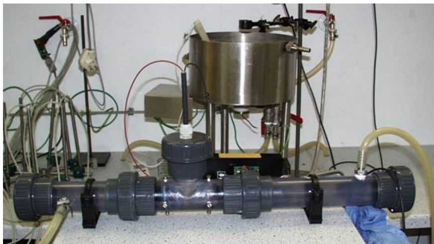
Figure 3 Ultrasonic Plasma Resonator (UPR) by USS (Test Facility), (Dorgeloh, Oliveri (2008))
