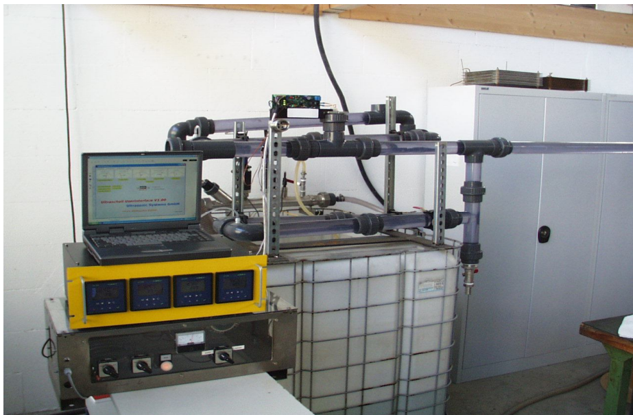
Figure 5 Test Facility for the Disinfection of Small Sewage Treatment Plant Waste Water (Dorgeloh, Oliveri (2008))
