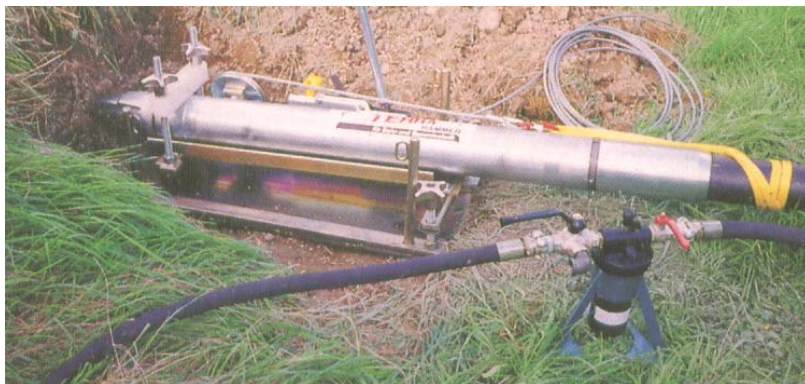
Figure 2. FORI 80 pneumatic rocket with the accessory kit
