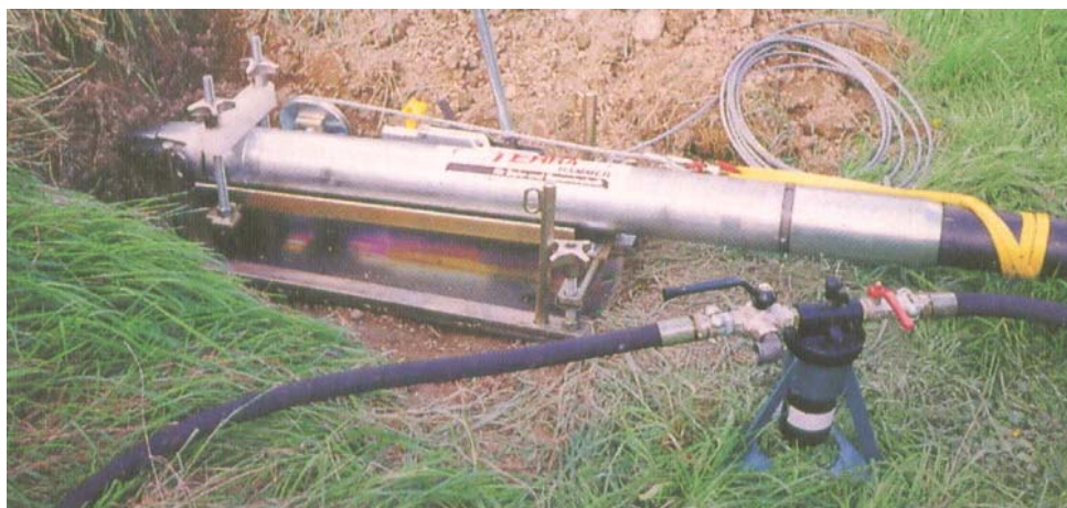
Figure 2. FORI 80 pneumatic rocket with the accessory kit
