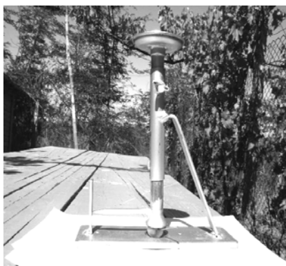
Fig.1. Device for determination of the deformation resistance of fruits (original)
