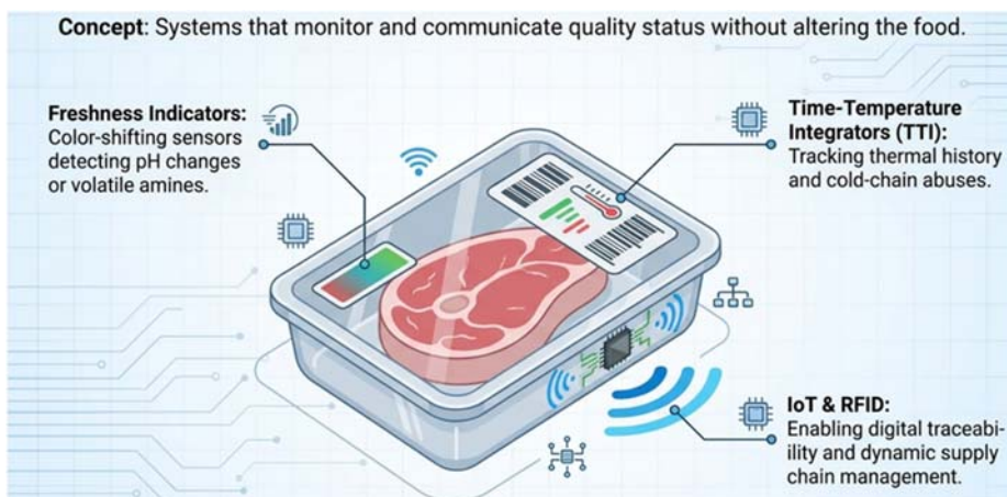
Fig. 2 .Illustration of intelligent packaging systems for real-time monitoring and traceability of refrigerated meat quality (created using NotebookLM and Canvas)
