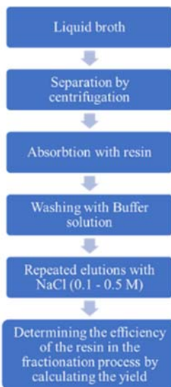
Fig. 3. Steps used for transglutaminase fractionation process
