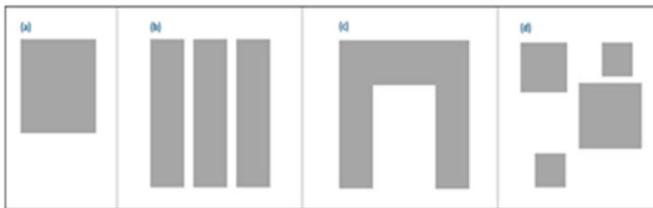
Fig. 1 Types of farm layouts. a) single building, b) identical large buildings placed in parallel, c) three-sided layout, d) scattered buildings. (Bucherer et al., 2021)
