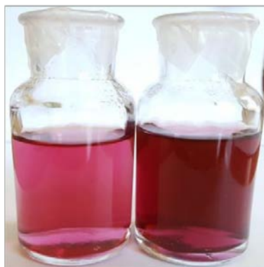
Fig. 1. AuNPs in chitosan solutions (different concentrations)
